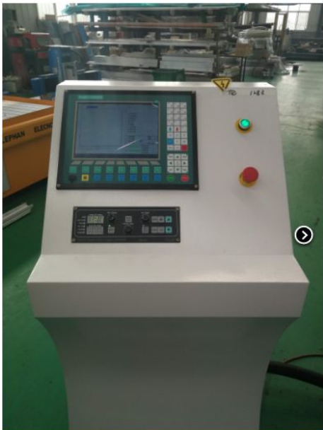
Fangling control system with THC (Anti-collision)
